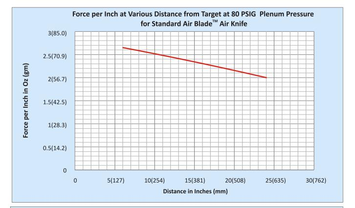
**NOTE:** Tests were preformed using a 12" Model 10012 Standard Air Blade<sup>™</sup> Air Knife
