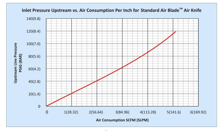
**NOTE:** Tests were preformed using a 12" Model 10012 Standard Air Blade $^{\text{TM}}$  Air Knife
