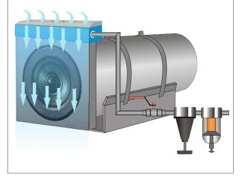
Two Model 10012 Standard Air Blade <sup>™</sup> Air Knives are installed on a duct (One on top, One on bottom) to draw in waste fumes & exhaust. The air leaving the Air Knives hug the inside wall creating an excellent vacuum inside the duct.
