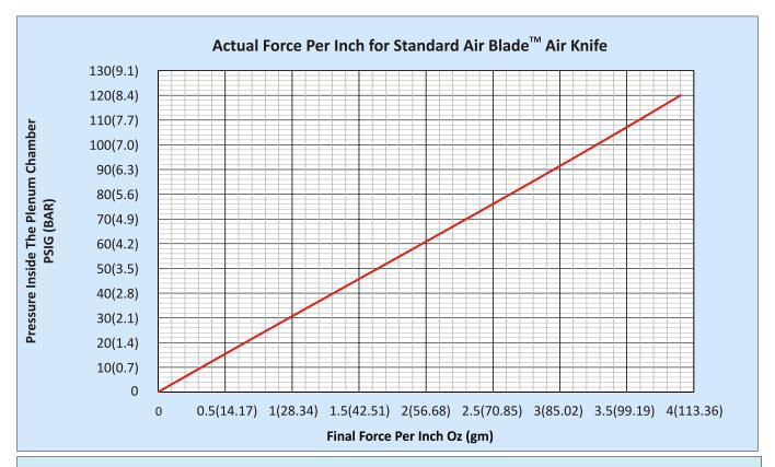
**NOTE:** Force per inch of Air Knife was based on tests done with a 12" Standard Air Blade<sup>™</sup> Air Knife with a .002" (.050 mm) gap. Force was measured at a target 6" from the Air Knife.
