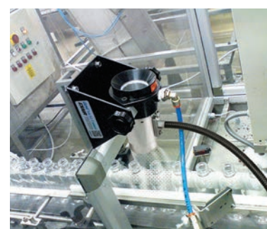
The Model 8292 Gen4 Ion Air Cannon System eliminates the static and dust prior to filling the bottles.
