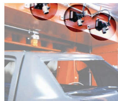
(3) Gen4 Ion Air Cannons blow contaminants from car bodies prior to painting.
