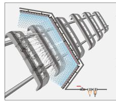
Three 24" X-Stream<sup>™</sup> Air Blade<sup>™</sup> Ionizers Blow off dust from Automotive Bumpers prior to painting. The NEX FLOW<sup>™</sup> PLCFC controls the air on and off as required minimizing air consumption. In this case the static bars were "daisy-chained" together minimizing extraneous cable and reducing the number of power supplies needed.
