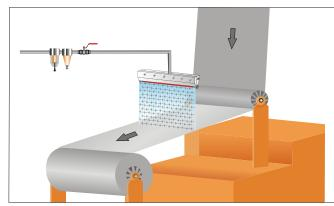
A Model 16118X removes static from extruded rubber web on a rewind. Previously the static charge was so high that any spark would cause the rubber to burn which regularly happens the 'extra strong' VS Bar combined with the X-stream Air Blade eliminated this unsafe situation.
