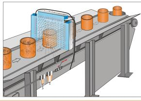
Three Model 15012 Standard Air Blade<sup>™</sup> Ionizer with 'extra strong' model VS static bar is used to remove the static charge from containers moving at high speed prior to filling. The Ionized air is blown in to the container to remove the static charge. All the static bars will connect with 4 outlet power supply. The VS Bars have to be used because of the high speed of container.
