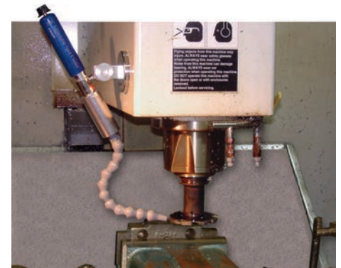
The Adjustable Spot Cooler replaces flood coolant and eliminates hours of cleanup on a cast iron machining operation.
