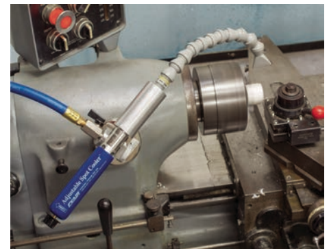
The Adjustable Spot Cooler maintains critical tolerances on machined plastic parts.
