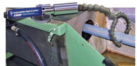
PVC hose is cooled at the exit of an extruder so it can be coiled immediately.
